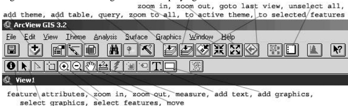
Figure 4. Menu and button guide when displaying a table in ArcView. The lower row represents the fields within the table, *Recno* is the active field.
